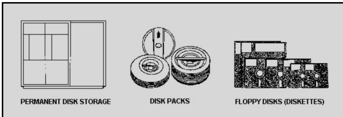
Figure 2-6 Various types and sizes of magnetic disk storage
