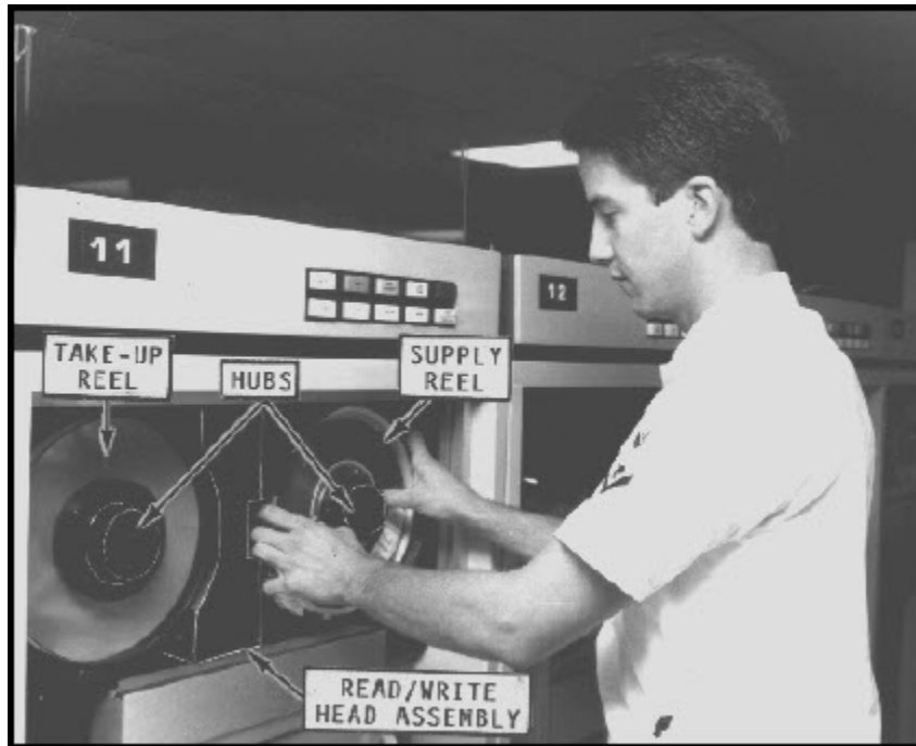
Figure 2-12 Mounting a magnetic tape
