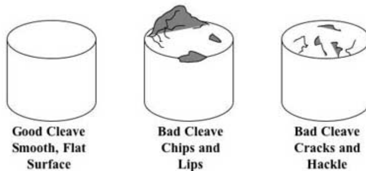
Figure 4-21. - Examples of Cleaves
