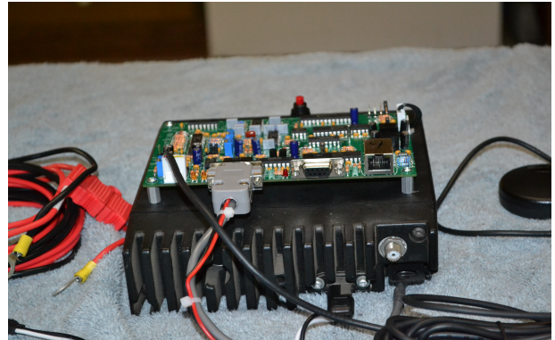
VOTER board shown installed on top of a Motorola Radius Receiver with GPS receiver and associated cabling
