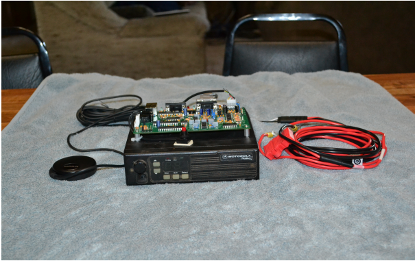
VOTER board shown installed on top of a Motorola Radius Receiver with GPS receiver and associated cabling
