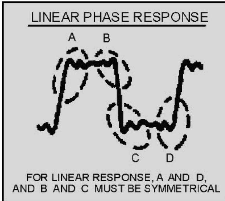
Figure 6-7 An example of good linear phase response
