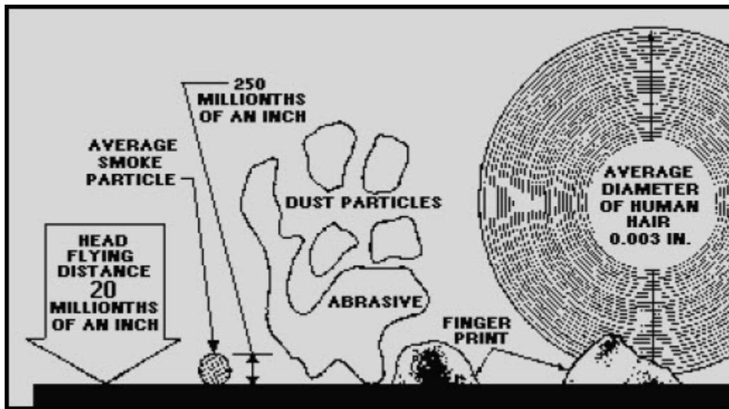
Figure 8-3 Size relationship of distance between head and disk to contaminants
