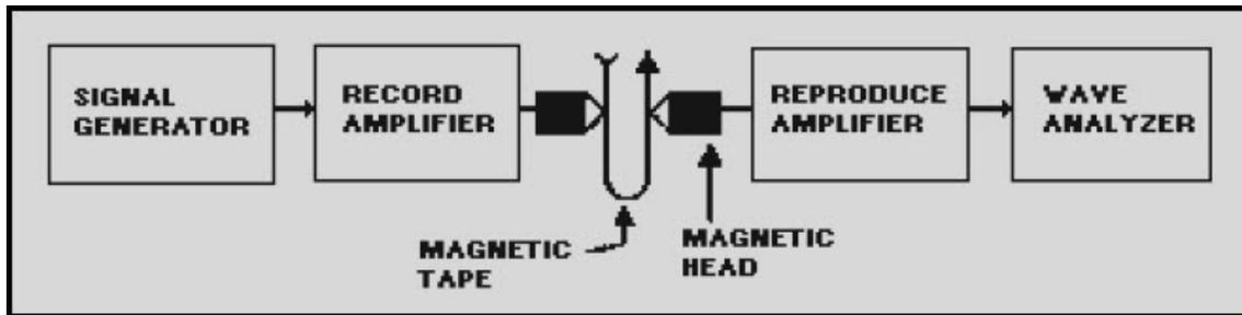
Figure 6-5 Test equipment setup for measuring harmonic distortion
