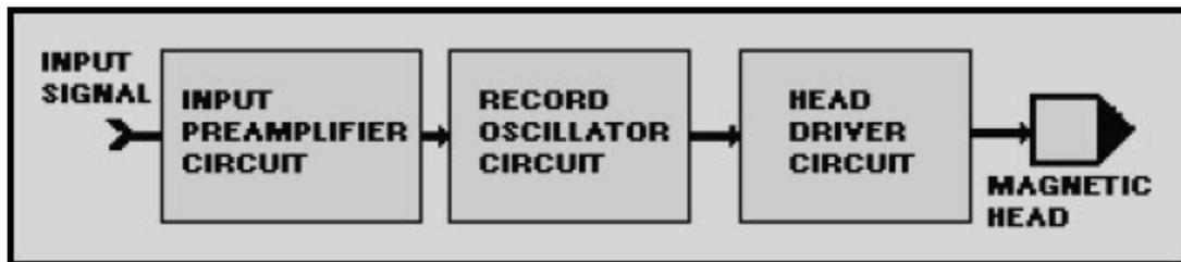
Figure 5-4 FM record electronics
