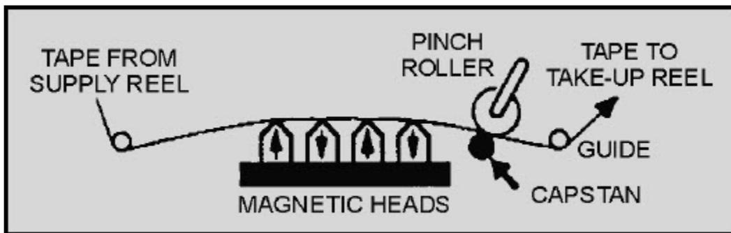
Figure 4-9 Open-loop capstan drive tape transport
