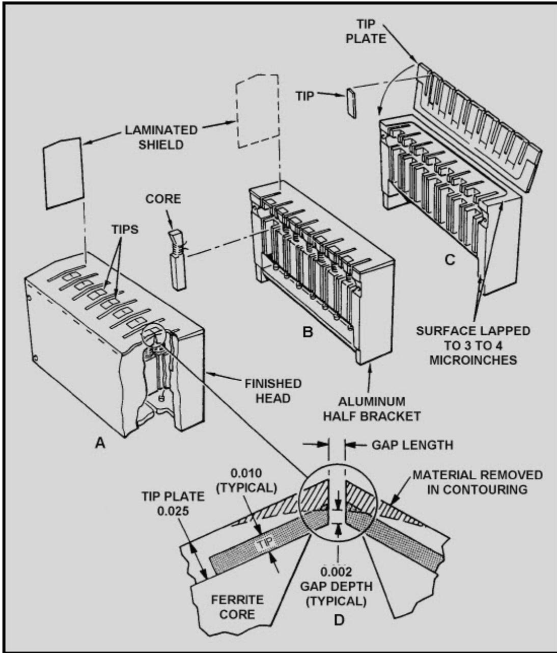
Figure 3-2 Multitrack tape recorder head construction
