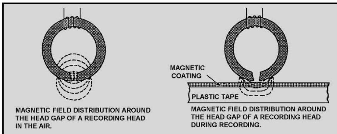
Figure 1-4 Magnetic field distribution around the head gap
